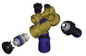
Convenient: The version with a stop valve has the advantage that once the isolating valve is closed, the backflow preventer and the pressure reducer cartridge can be cleaned or replaced – without having to drain the installation.
